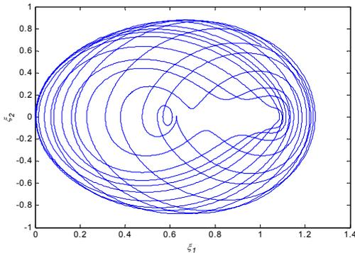
Figure 2 Phase Plot of the System Response for  $\mu(t) = 0.6 + 0.5\sin(2t + \frac{\pi}{2})$
