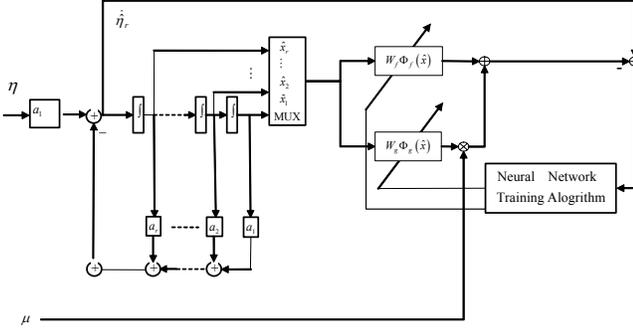
Figure 1 On-line System ID from I/O Data
