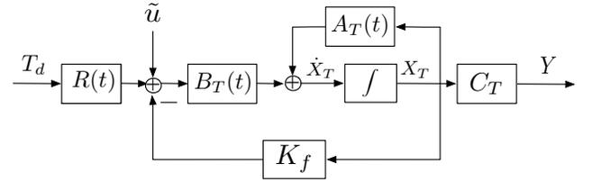
Fig. 2. The full-state feedback  $K_f$  stabilizes the tension loop. Time-varying  $R(t)$  takes into account the time-varying nominal radius and  $\tilde{u}$  is the feedforward input to address reel eccentricities.
