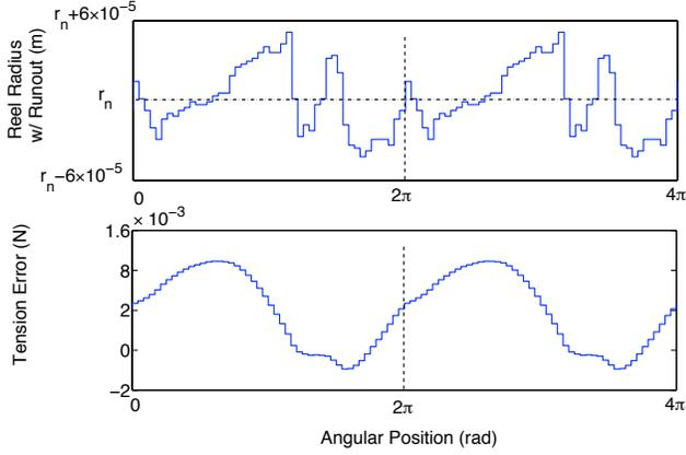
Fig. 3. Periodic reel runout and the tension error due to the runout for two revolutions.
