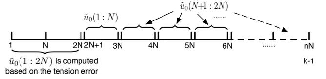
Fig. 4. Two periods of tension error signal are used to compute the compensation input series.
