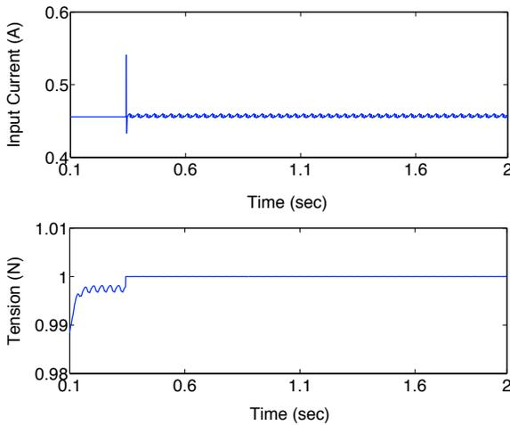
Fig. 11. The time-varying input attenuates the tension error by 3 orders of magnitude.
