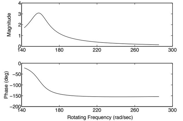
Fig. 5. Magnitude and phase of the time-varying  $G_T$  as a function of the time-varying reel radius evaluated at the corresponding rotating frequency.
