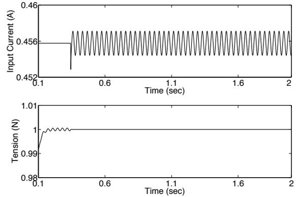
Fig. 9. Tension error is reduced after the compensation input is applied.
