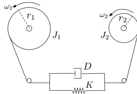
Fig. 1. Lumped-parameter model of a tape system.
