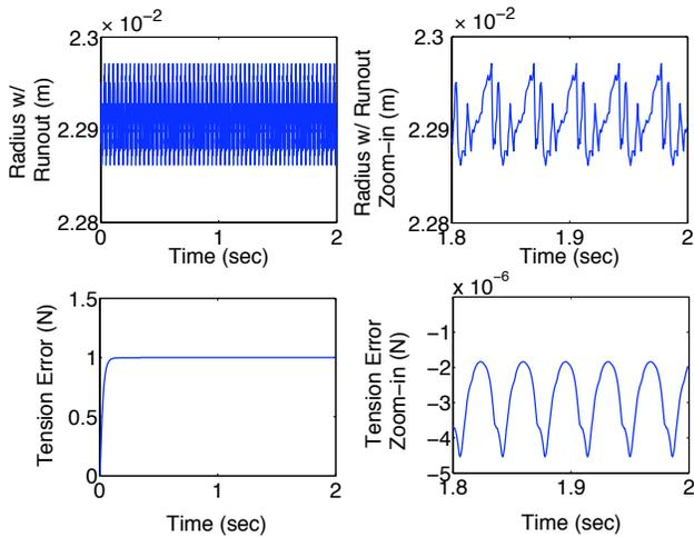
Fig. 10. Results using reel runout data from a tape manufacturer. The period of the residual tension error is the same as that of the runout.
