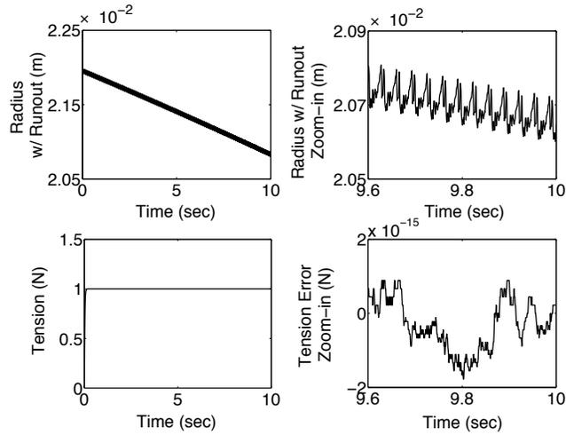
Fig. 7. Tension error is eliminated by a time-varying reference input that addresses both nominal reel radius variations and runout.
