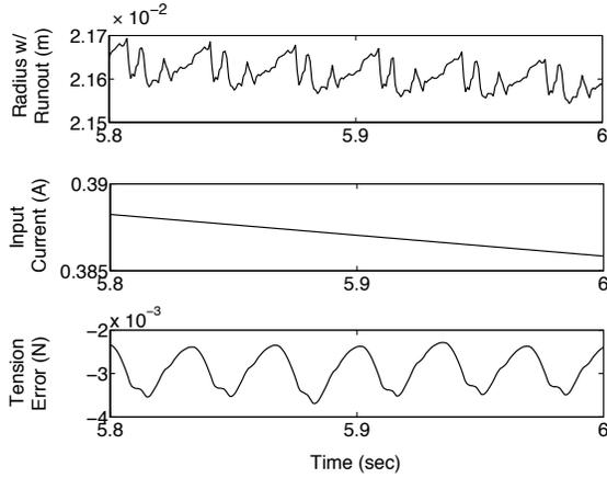
Fig. 6. The reel runout is from a tape manufacturer. The input current does not account for reel eccentricities and the tension error is on the order of  $10^{-3}$  N.
