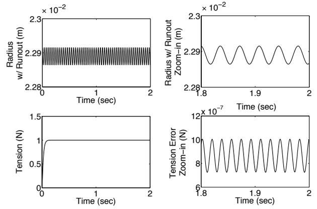
Fig. 8. Sinusoidal reel runout causes sinusoidal tension error; the compensation input is sinusoidal as well. The frequency of the residual tension error is twice that of the runout.
