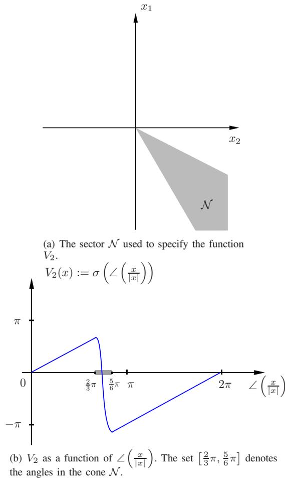
Fig. 4. Function  $V_2$  for the application of Theorem 3.2 to the non-Zeno bouncing ball system.
