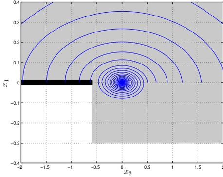
(b) After a finite number of jumps, the ball's trajectory remains in the flow set and asymptotically converges to  $\mathcal{A}$  by only flowing.
