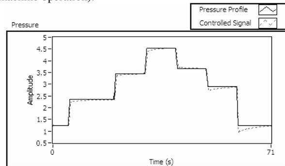
Fig. 9. Pressure profile and controlled simulation for increasing and decreasing vacuum.
