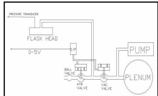
Fig. 1. Schematic diagram of counter-gravity machine with single controller.
