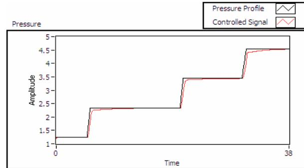
Fig. 8. Controlled simulation for a 0.5s span step input.
