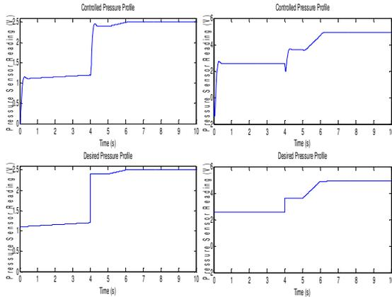
Fig. 6. The desired and the controlled pressure at two different regions: (a) First TF in Table 3 & (b) Fourth TF in Table 3
