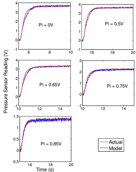
Fig. 2. The response of the model compared with the response of the actual system: 0.5 in vacuum valve stem position with different initial vessel pressures.
