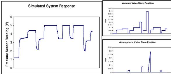
Fig. 5. The response of the simulated system with vacuum and atmospheric valve stems position as input.
