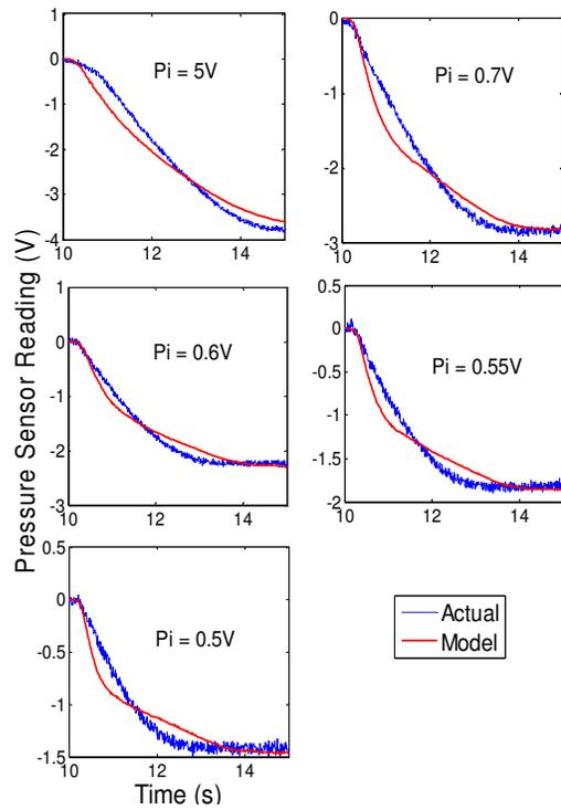
Fig. 3. Model and actual system response: 0.3in atmospheric valve stem position with different initial vessel pressures.
