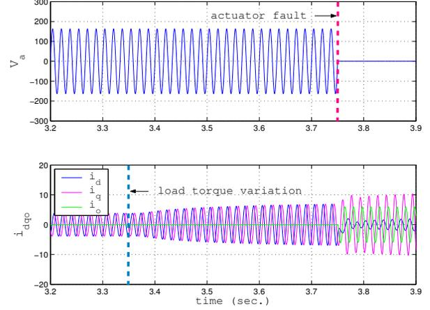
Fig. 1. Simulation Results Case A: (TOP) Phase-*a* Voltage, (BOTTOM) Line currents in *dqo*-frame.
