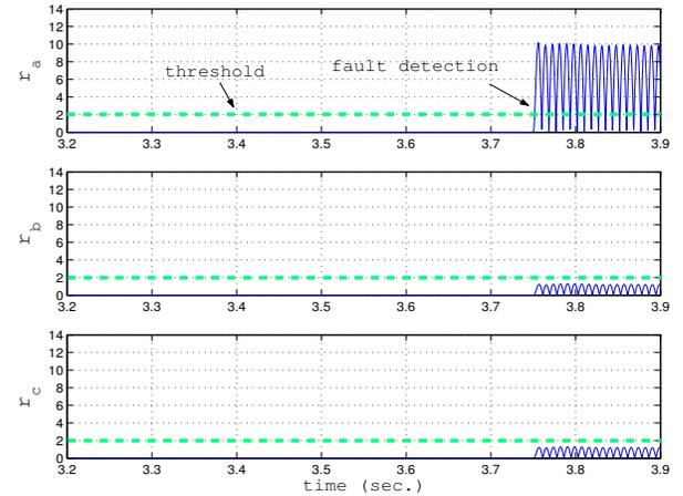
Fig. 2. Simulation Results Case A: Residuals (TOP) Phase-*a*, (MIDDLE) Phase-*b*, and (BOTTOM) Phase-*c*.
