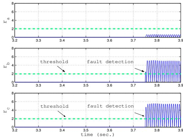
Fig. 4. Simulation Results Case B: Residuals (TOP) phase-a, (MIDDLE) phase-b, and (BOTTOM) phase-c.
