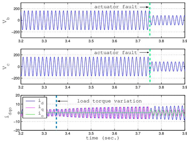
Fig. 3. Simulation Results Case B: (TOP) Phase-b voltage, (MIDDLE) Phase-c voltage, and (BOTTOM) Line currents in  $dqo$ -frame.
