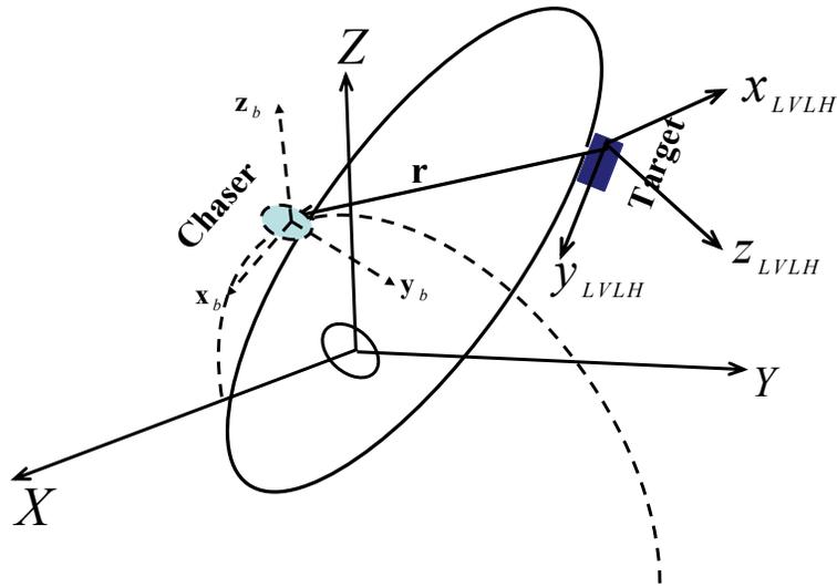
Fig. 1. The LVLH and Body Frame
