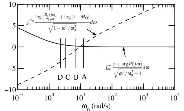
Fig. 4: Right and left sides of the inequality in Proposition 1 for  $M_\Theta = 0.5$ . Lines A, B, C, and D indicate four specification for  $\omega_c$ .
