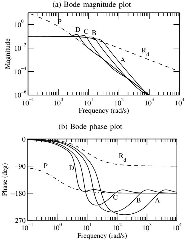
Fig. 6: Frequency response of the haptic device  $P$ , the virtual environment  $R_d$ , and four causal approximations to  $R_d$  (designs A, B, C, & D). Designs A, B, and C violate passivity since their phase drops below -180 degrees.
