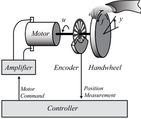
Fig. 1: Schematic of a rotary haptic device and controller.
