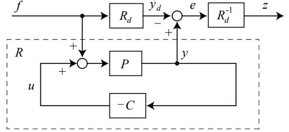
Fig. 2: General control configuration for haptic rendering with position feedback. The closed-loop response from  $f$  to  $z$  is given by distortion  $\Theta$ .
