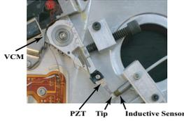
Fig. 2. The dual-stage actuator experimental system.
