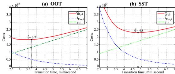
Fig. 3. Comparison of time/input-energy cost: OOT vs SST.
