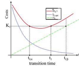
Fig. 1. Schematic sketch of transition-time cost  $\gamma t_f$ , energy cost  $J_{E,opt}$  and total time/energy cost  $\hat{J}(t_f)$  as functions of transition-time  $t_f$ .
