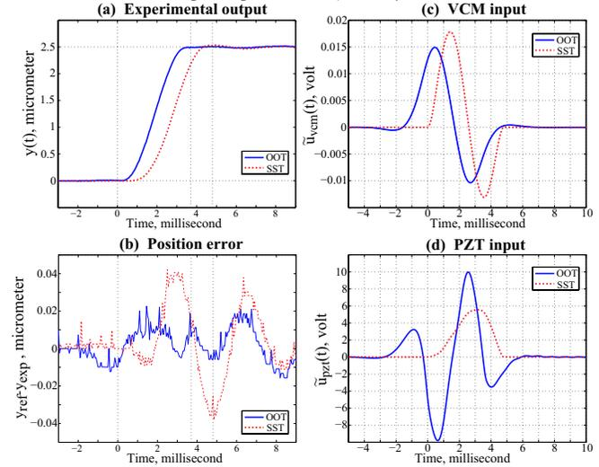
Fig. 4. Experimental results for 2.5-micrometer output-transition: (a) Output trajectory, (b) Position error with OOT approach, (c) VCM-input trajectory, and (d) PZT-input trajectory.
