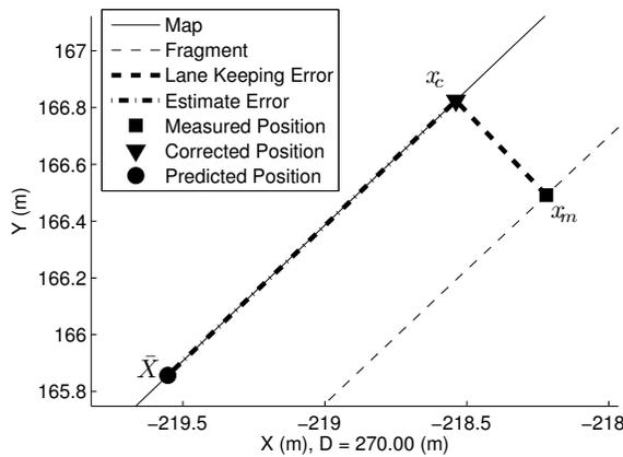
Fig. 6. Lane keeping error and its correction.
