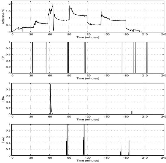
Fig. 2. Isoflurane and stimuli inputs versus time
