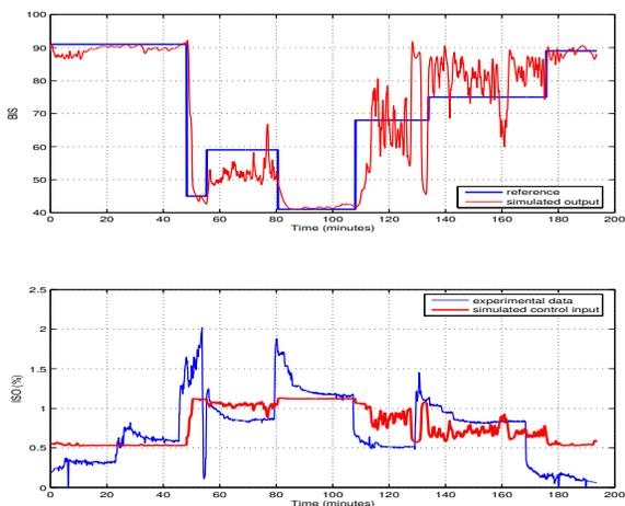
Fig. 6. Control simulation result of BIS reference tracking for volunteer 1
