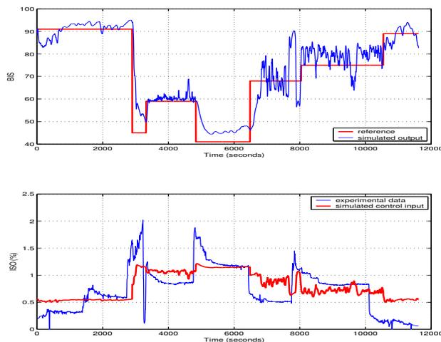
Fig. 8. Patient 3 controller with patient 1 model/data for BIS reference tracking
