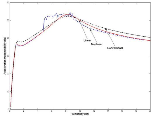
Fig. 4 Acceleration transmissibility of the nonlinear, linear and conventional models
