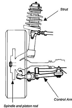
Fig. 1. Schematic of Macpherson Strut Suspension
