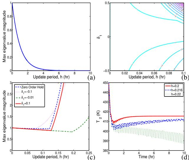
Fig. 2. Dependence of  $\lambda_{max}$  on (a) the update period using accurate models, and (b) on plant-model mismatch for various update periods. Plot (c): Maximum stabilizing update period using different compensating models and a zero-order hold scheme. Plot (d) shows the closed-loop profiles of  $T_2$  with  $\delta_1 = -0.01$  for different update periods.
