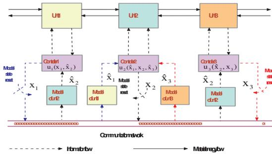
Fig. 1. Model-based quasi-decentralized control of a plant of interconnected units over a communication network.
