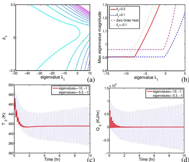
Fig. 3. Plots (a)-(b): Dependence of  $\lambda_{\max}$  on local feedback controller gain,  $K_1$ , with different model uncertainties. Plots (c)-(d): Closed-loop state and manipulated input profiles with  $h = 0.1$  hr and  $\delta_1 = 0.2$  for different feedback gains  $K_1$ .
