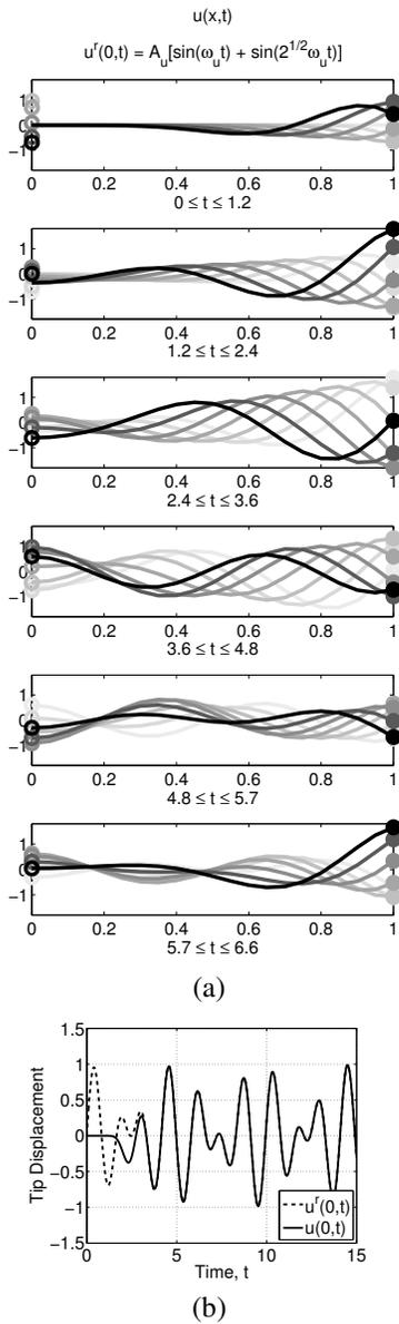
Fig. 2. String simulation results showing (a) the string state as snapshots in time, and (b) a comparison of the string tip displacement and reference trajectory.
