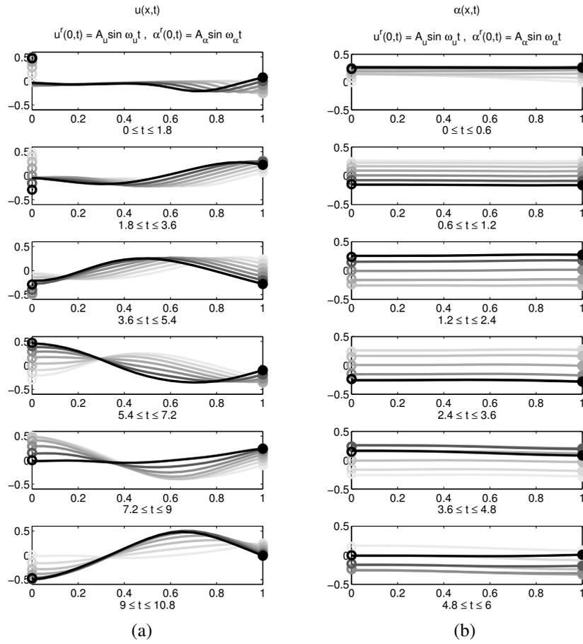
Fig. 3. Shear beam simulation results showing snapshots of the beam states (a)  $u(x, t)$ , and (b)  $\alpha(x, t)$  for simultaneous reference tracking.
