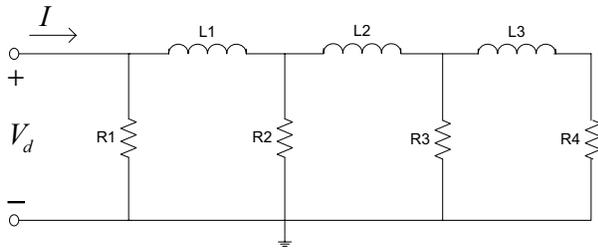
Fig. 2. RL circuit network
