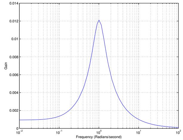
Fig. 5. Closed loop bode plot with stable positive real controller.
