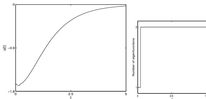
Fig. 3. (a) Profile of the magnitude of actuation for distributed control action, (b) Number of empirical eigenfunctions (also the order of the reduced ODE model) as a function of time for distributed control action.
