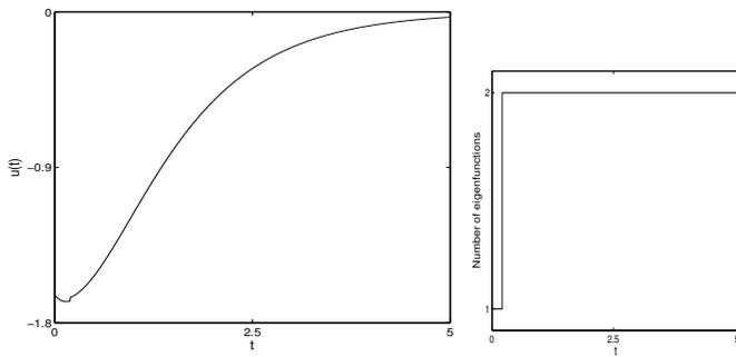
Fig. 7. (a) Profile of the magnitude of actuation for point control action, (b) Number of empirical eigenfunctions (also the order of the reduced ODE model) as a function of time for point control action.
