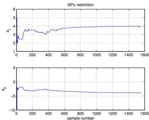
Fig. 8. Profiles of the coefficients  $a_1$  and  $a_2$  vs. the sample number for 95% restriction
