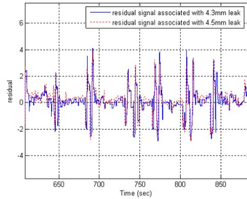
Fig. 3. The EGR mass flow residual signal calculated using actual measurement and output of the adapted healthy system
