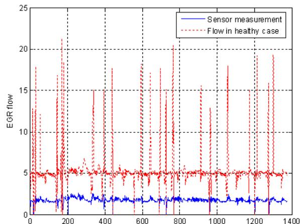
Fig. 5. The EGR mass flow in the low flow faulty condition and the amount of gas that should have flowed through the EGR passage
