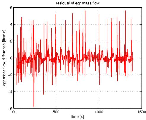
Fig. 2. The EGR mass flow residual signal generated using the measurement and output of the adapted model
