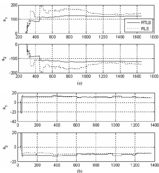
Fig. 4. Results of the parameter identification using the RLS and RTLS algorithms: (a) baseline and (b) restricted condition
