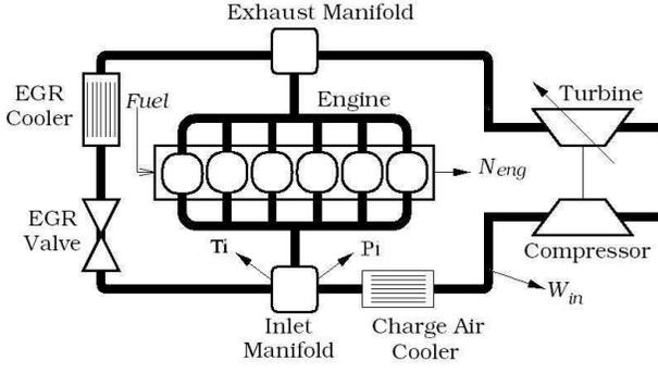
Fig. 1. Simplified schematic view of the airpath in a Diesel engine [12]
