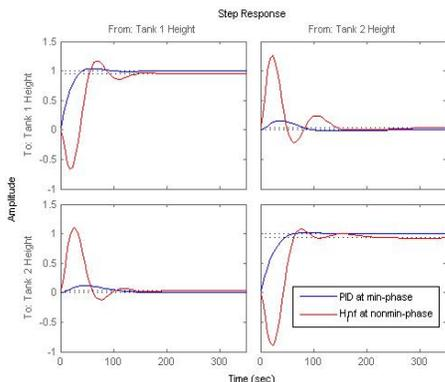
Figure 5: Step response of PID controller at minimum phase design point
