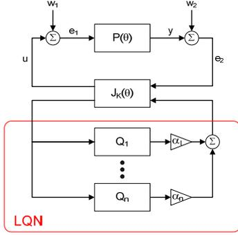
Figure 2: Output Blending of Local Q-Network (LQN)
