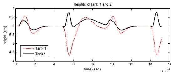
Figure 9: Fluid heights in lower tanks for gain scheduled controller (disturbance rejection due to changes in  $\gamma_1 / \gamma_2$ )
