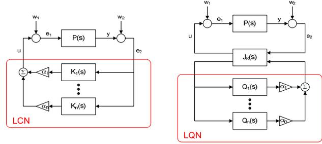
Figure 1: Output Blending of Local Controller Network (LCN) and Local Q-Network (LQN)
