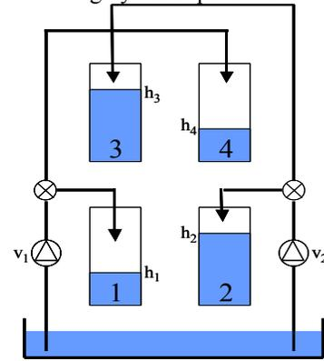
Figure 3: Diagram of a Quadruple Tank System
