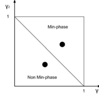
Figure 4: Controller design points in minimum and non-minimum phase region due to gamma values
