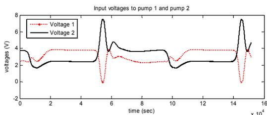
Figure 8: Control input voltages to pump 1 and 2
