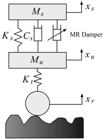
Fig. 1. Suspension system with MR damper
