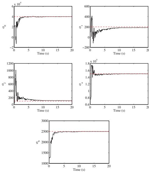
Fig. 7. Convergence of MR parameter estimates for skyhook control with forward modeling.
