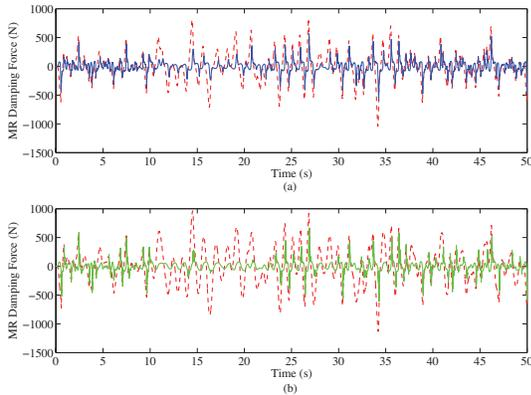
Fig. 8. Plot of  $F_A$  (red, dashed) and  $F_{MR}$  versus time for (a) skyhook control with forward modeling (blue, solid) and (b) skyhook control with inverse modeling (green, solid).
