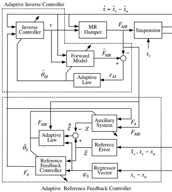
Fig. 2. Proposed fully adaptive semi-active control scheme based on forward modeling
