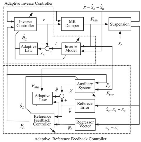
Fig. 3. Proposed fully adaptive semi-active control scheme based on inverse modeling
