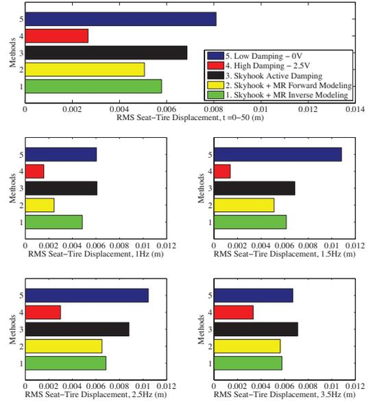
Fig. 5. Comparison of RMS seat-tire displacement for the entire simulation, and divided into different frequency ranges.
