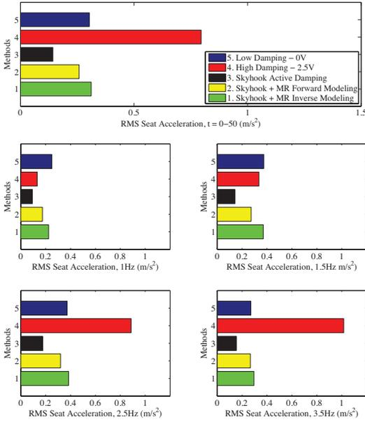
Fig. 4. Comparison of RMS seat acceleration for the entire simulation, and divided into frequency ranges.
