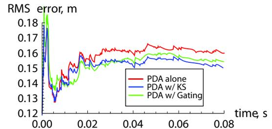
Fig. 5. RMS errors for PDA with the KS test, PDA with gating, and PDA alone when two cars are moving 10m apart.
