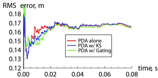
Fig. 6. RMS errors for PDA with the KS test, PDA with gating, and PDA alone when two cars are moving 2m apart.
