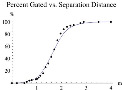
Fig. 2. Percent of incorrect measurements correctly gated out. The points are data points obtained by varying the separation distance between the two cars; the solid line is a curve fit to the data.
