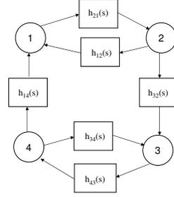
Fig. 2. Network topology: four agents with six channels.
