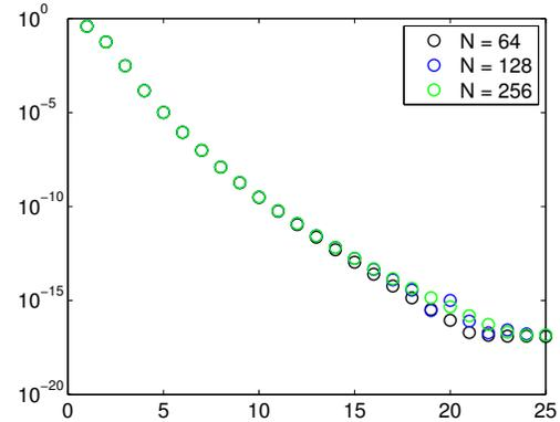
Fig. 1. POD eigenvalues computed using  $N = 64, 128$ , and  $256$  equally spaced finite element nodes.
