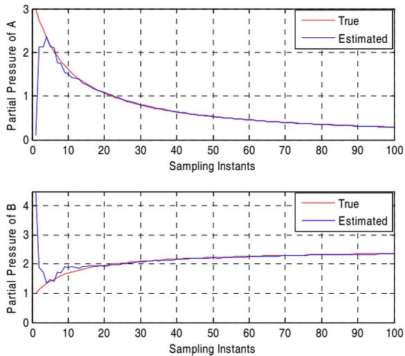
Figure 1: Evolution of true and estimated states of Partial pressures in Gas-phase reactor (CEnKF)
