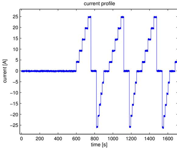
Fig. 3. Current profile designed to excite the battery.
