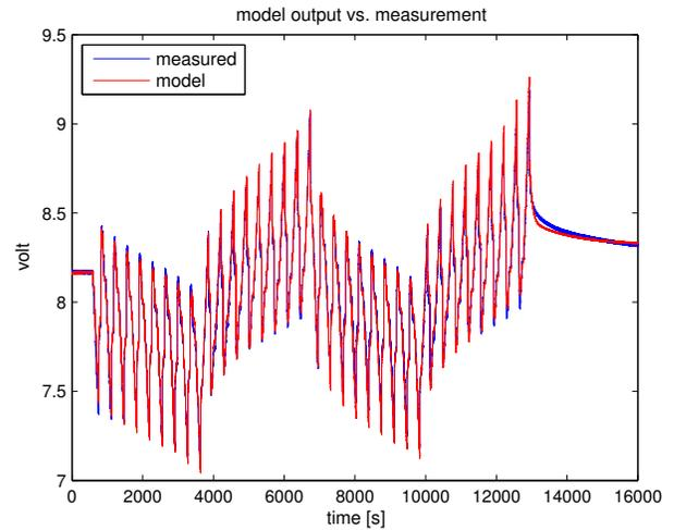
Fig. 11. Validation of the constant parameter model with OCV curves optimized by GA; average error = 0.022 V
