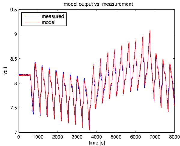
Fig. 9. Battery voltage from the LPV model with OCV curves modified by GA vs. measured battery voltage; average error = 0.020 V
