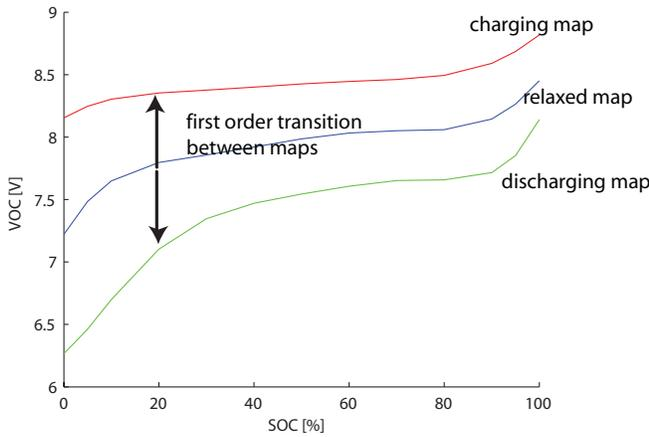
Fig. 2. Transition between different maps modeled by 1st order system
