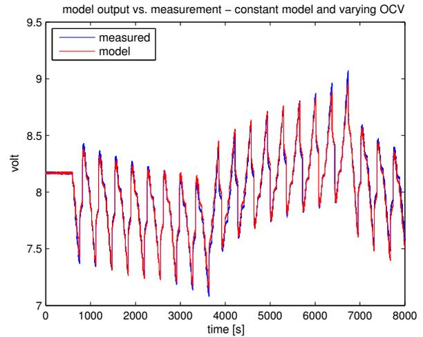
Fig. 7. Battery voltage from constant model with GA optimized OCV curves vs. measured voltage; average error = 0.028 V
