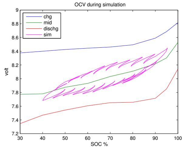
Fig. 8. Modified OCV curves in the second identification, where model parameters are constants
