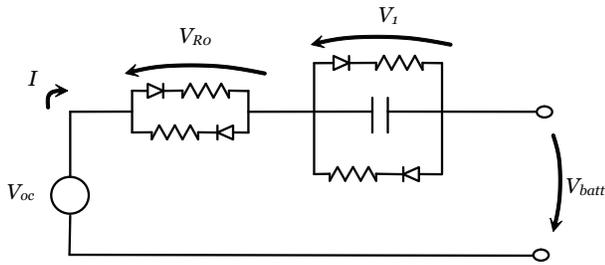
Fig. 1. Electrical circuit model of battery
