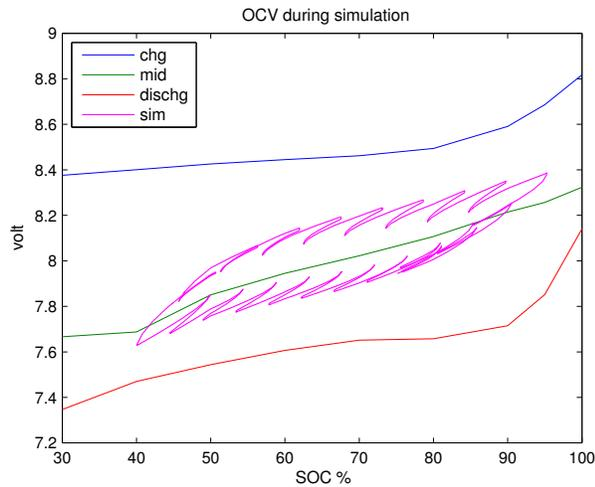
Fig. 10. OCV curves modified by GA in this identification
