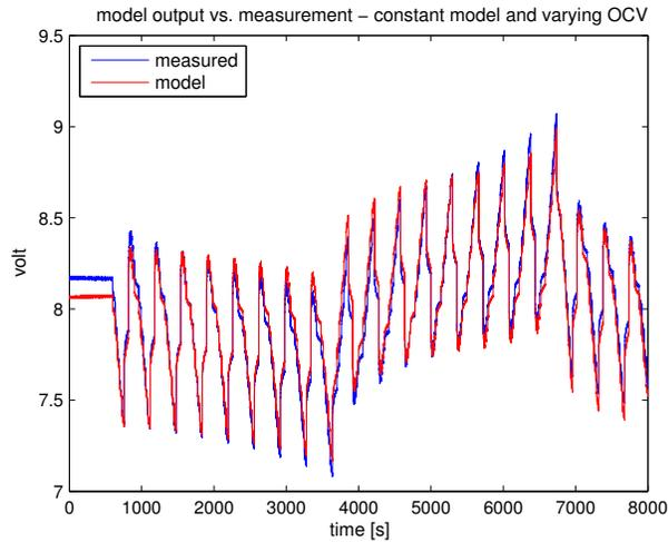
Fig. 5. Battery voltage from constant model with experimental OCV curves vs. measured voltage; average error = 0.055 V
