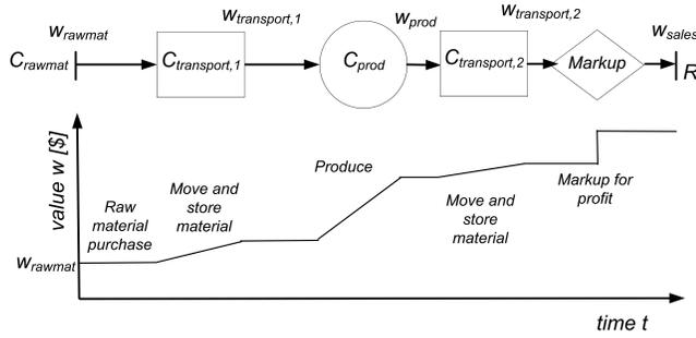
Fig. 2. The value chain tracks how process operations add value to goods as they move through the production system. The last section includes the price markup as a value added step.
