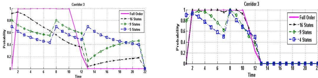
Fig. 6. Estimation results with spectral (left) and entropy (right) methods: the plots show the estimate probabilities of being located in Corridors 3. Full order estimation as well as reduced order estimation using a varying number of super-states are displayed.
