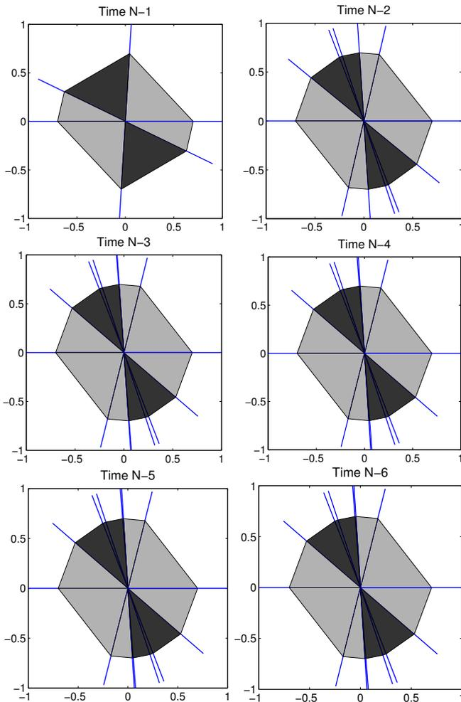
Fig. 2. Switching Regions for Ex1: Gray Region – mode 1 optimal; Black Region – mode 2 optimal.
