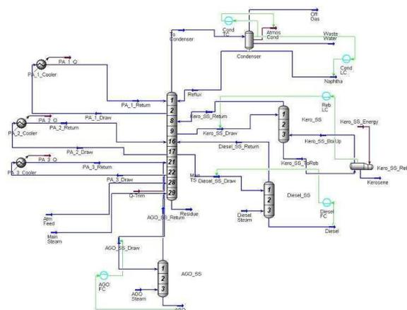
Fig. 1. A dynamic HYSYS distillation plant simulation flow sheet.
