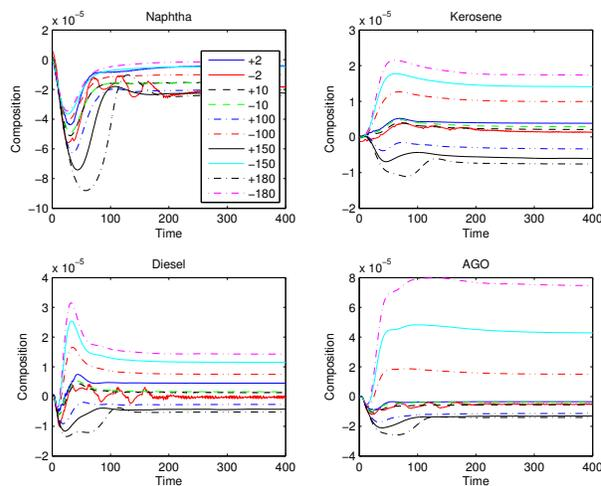
Fig. 3. Normalized output response for Reflux flow step changes.
