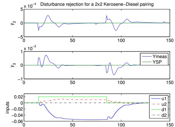
Fig. 9. Disturbance rejection for a 2x2 control, normalized Kerosene and Diesel compositions
