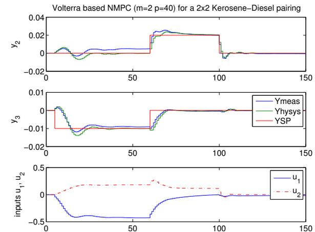
Fig. 10. Closed-loop nonlinear MPC 2x2 control, normalized Kerosene and Diesel compositions
