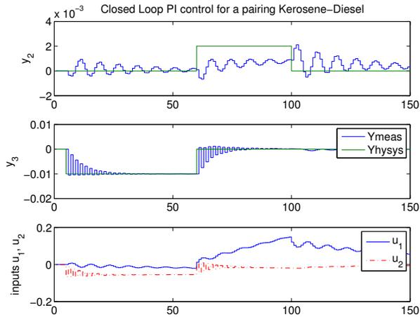
Fig. 7. PI control of a nonlinear interacting pairing (kerosene-diesel).
