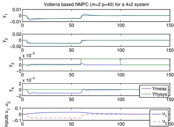
Fig. 8. Nominal nonlinear MPC closed-loop control showing setpoint tracking.  $m=2$ ,  $p=40$ ,  $\Gamma_y = [10 \ 10 \ 10 \ 10]$ ,  $\Gamma_{\Delta u} = [1 \ 1]$ .
