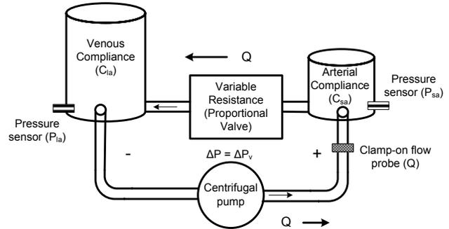
Fig. 3. Schematic of MCS, showing sensors and actuators, where  $Q$  represents the cardiac output  $CO$ .
