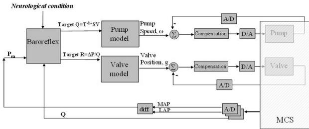
Fig. 4, Block diagram of the control scheme
