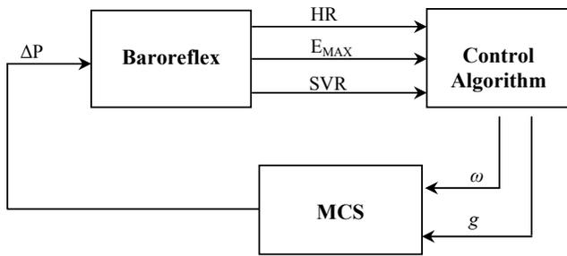
Fig. 2. Block diagram of the baroreflex control of the MCS
