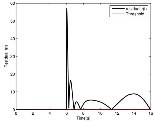
Fig. 2. Detection of abrupt sensor faults
