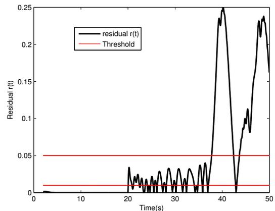
Fig. 3. Detection of incipient actuator faults
