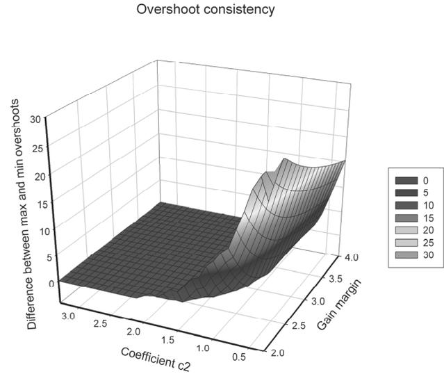
Fig. 6. Difference between maximum and minimum overshoot [%] for modified RFT
