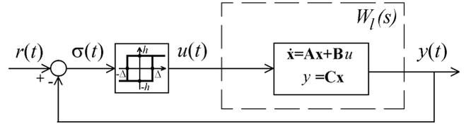
Fig. 3. Relay feedback test
