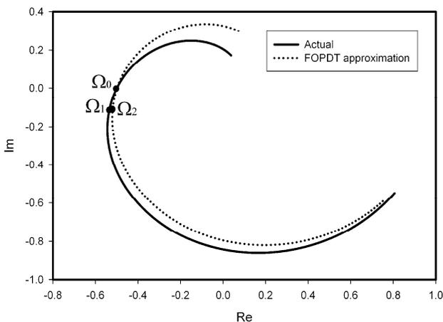
Fig. 1. Nyquist plots for process (1) and FOPDT approximation (3)
