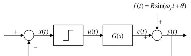
Fig. 1. Single loop with external forcing signal.
