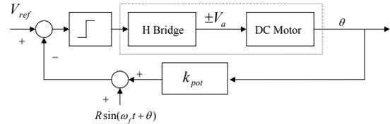
Fig. 12. Model of the DC motor in example 6.
