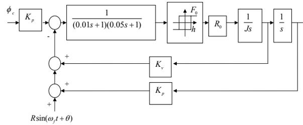
Fig. 9. Block diagram of the Missile Roll-Control problem. [14]
