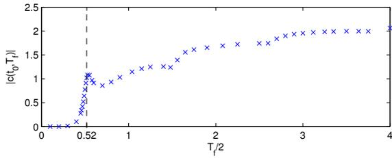
Fig. 2. Plot of the amplitude of oscillation against  $T_f/2$  for  $G(s) = 1000/(s^5 + 6s^4 + 58s^3 + 211s^2 + 629s + 471)$ .
