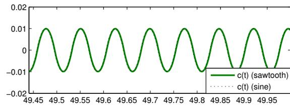
Fig. 11. Plot of  $c(t)$  with sine and sawtooth dither
