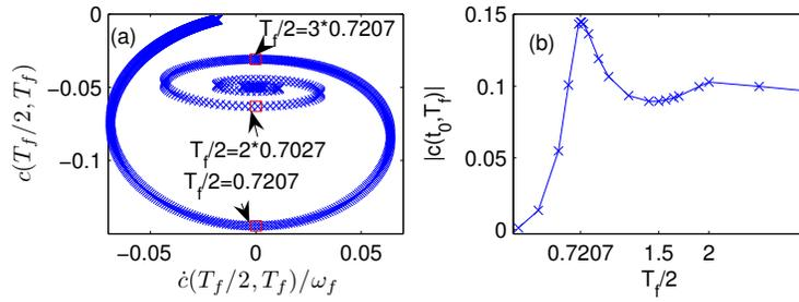
Fig. 7. (a)Plot of the Tsytkin Locus in example 3. (b)Plot of the amplitude of oscillation against  $T_f/2$  in example 3.
