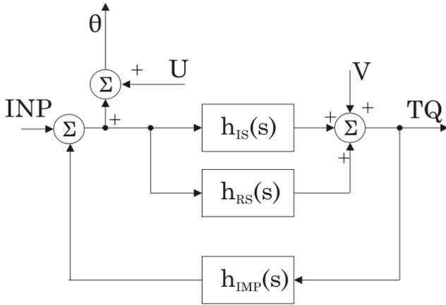
Figure 2. Simplified block diagram of the closed-loop ankle-actuator system.  $H_{imp}(s)$  represents dynamics of the impedance controller.  $H_{IS}(s)$  and  $H_{RS}(s)$  represent transfer functions for intrinsic and reflex stiffness. INP, TQ and  $\theta$  represent input perturbation, torque and position signals. U and V represent torque and position error signals.
