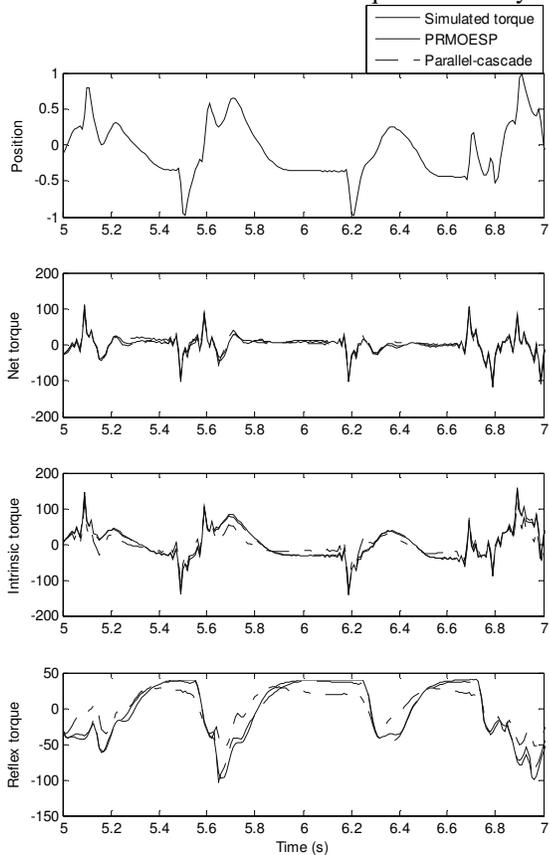
Figure 3 Comparison of estimated and observed torques
