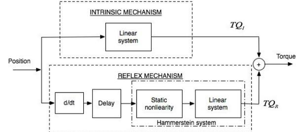
Figure 1 Parallel-cascade structure of ankle dynamics.  $TQ_i$  and  $TQ_r$  denote intrinsic torque and reflex torque. The position signal is the input signal to the parallel-cascade method, while the torque signal, the sum of the intrinsic and reflex torques, is the measured output. Intrinsic stiffness is modeled as a linear system. Reflex stiffness is modeled by a series connection of a differentiator, a delay, a static nonlinearity and a linear low-pass system.
