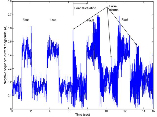
Fig. 1. Negative sequence current for (unloaded and fault condition ( $0 < t < 6.5$  sec) and load fluctuation and fault condition ( $t > 6.5$  sec)).
