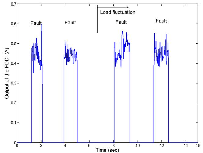
Fig. 5. Output of the FDD purposed (Loop current 25 A. 0-30% load)
