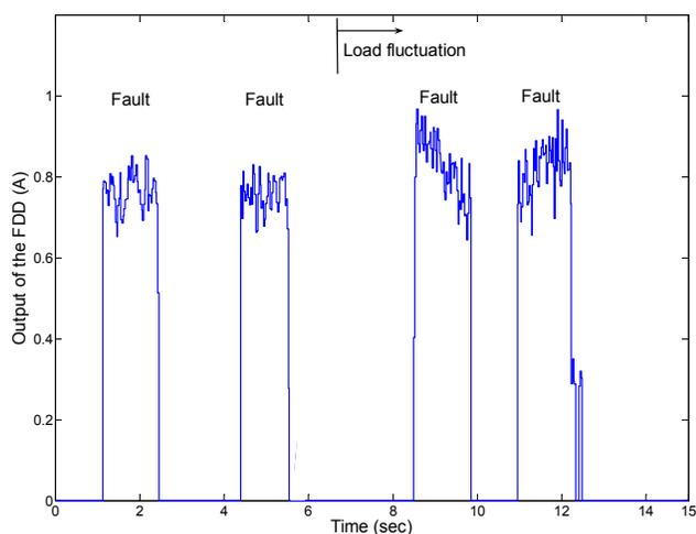
Fig. 7. . Output of the FDD purposed (Loop current 41.5 A. 0-45% load)
