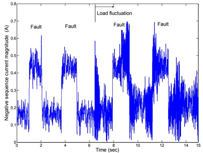
Fig. 4. Negative sequence current (Loop current 25 A. 0-30% load).
