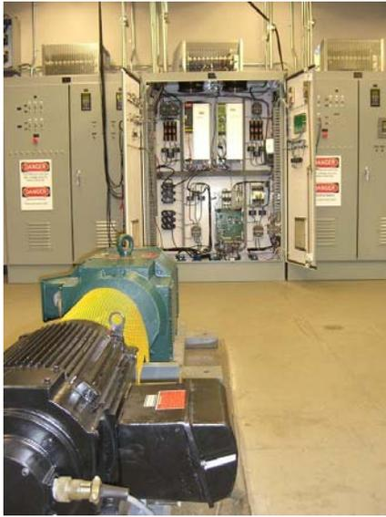
Fig. 3 Completed electrical experimental setup.
