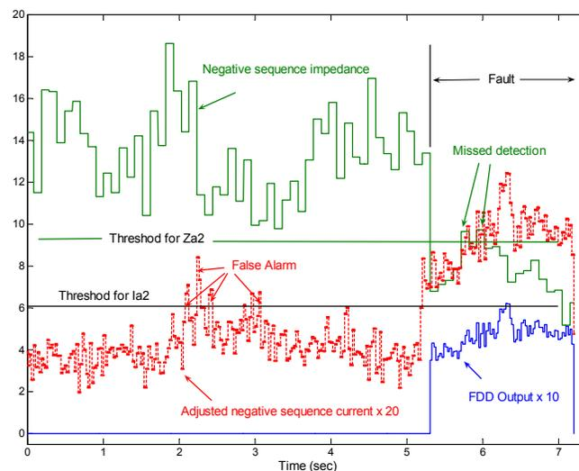
Fig. 8. Proposed FDD method versus negative sequence current/impedance
