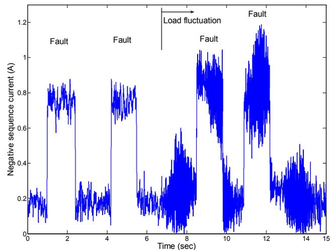
Fig. 6. Negative sequence current (Loop Current 41.5 A. 0-45% load)
