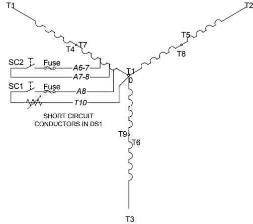
Fig. 4. Stator winding short circuit setup with external variable resistor
