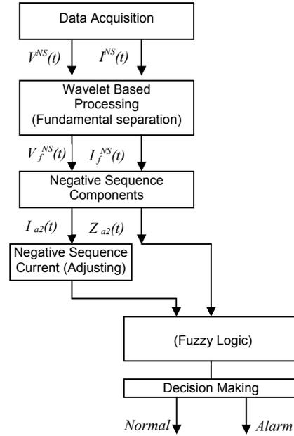
Fig. 2. Schematic diagram of the detection process
