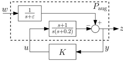
Fig. 6. Closed-loop layout.
