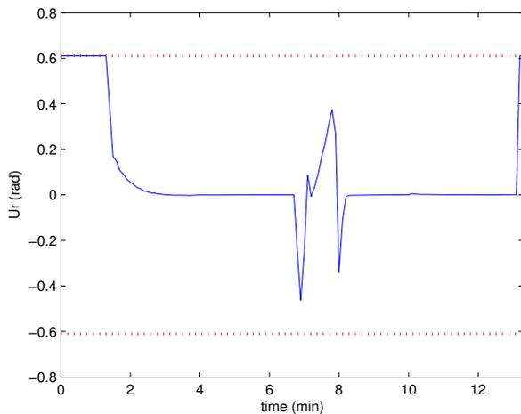
Fig. 3. Time history of the rudder angle. Dashed lines indicate constraints.
