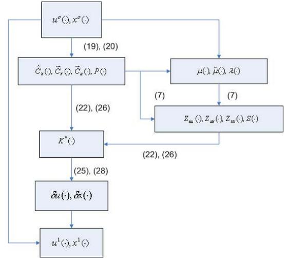
Fig. 1. Computation sequence for calculating the neighboring extremal solution.
