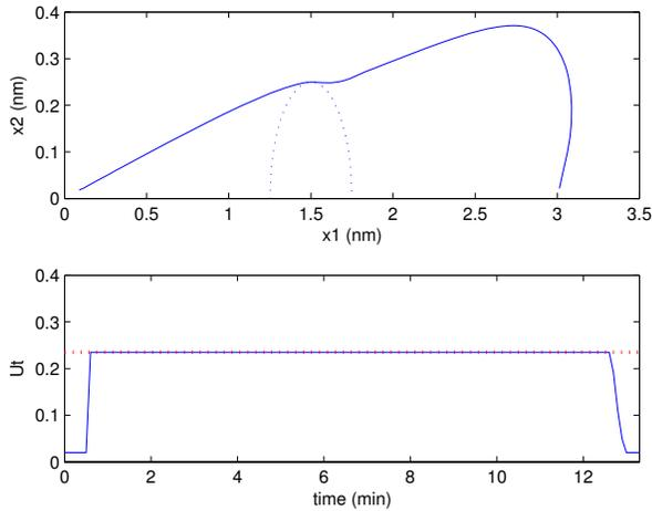
Fig. 2. Ship position on  $x_1$ - $x_2$  plane (top) and time history of the propeller thrust (bottom). Dashed lines indicate constraints.
