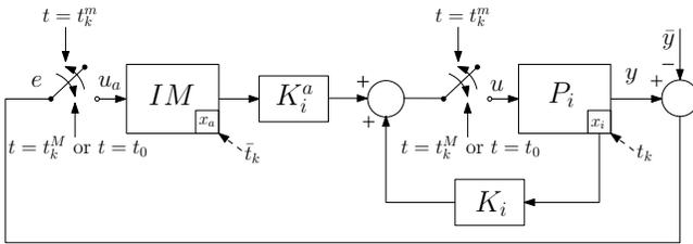
Fig. 2. Structure of the control scheme based on the internal model principle with switching control laws (14) and (15).
