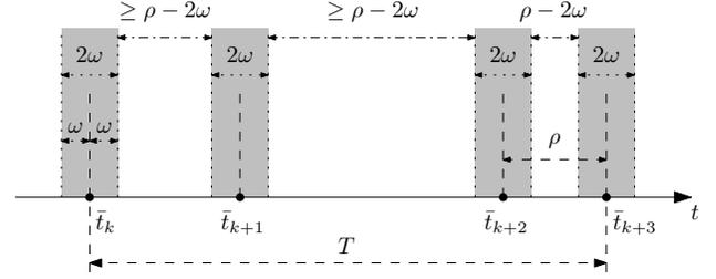
Fig. 1. Example of possible switching times for a trajectory with period  $T$  and  $N = 3$  switching events per period. Time intervals identified by the grey blocks are neglected in the stability analysis.
