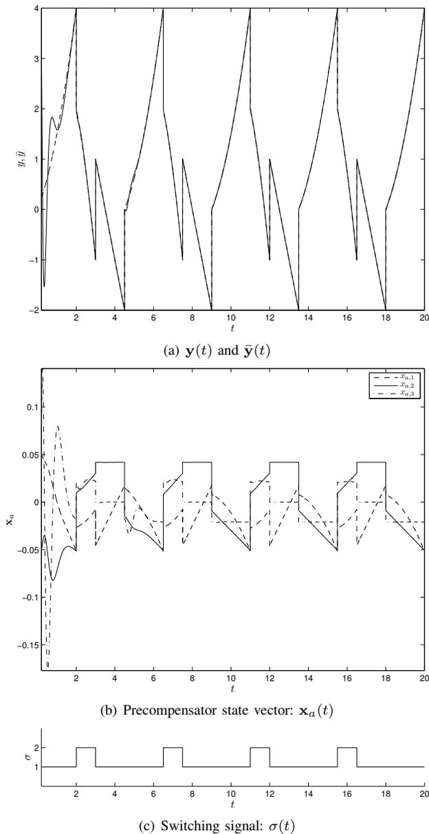
Fig. 4. The desired (dashed) trajectory and the actual (solid) one (a); time behavior of the precompensator state variables  $\mathbf{x}_a(t) = [x_{a,1} \ x_{a,2} \ x_{a,3}]^T$  (b); switching signal relevant to the controlled trajectory (c).
