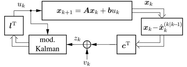
Figure 2. Proposed scheme with innovation coding and modified Kalman filter for noiseless system ( $\mathbf{w}_k \equiv \mathbf{0}_M$ ).
