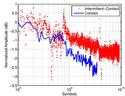
Fig. 8. Normalized average signal amplitude (dB scale) during an intermittent-contact and contact read experiment.
