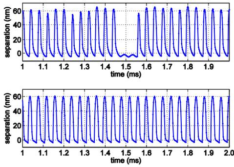
Fig. 4. Read-back signals from an intermittent-contact experiment (bottom) with and (top) without feedback. Without the feedback loop, the cantilever adheres to the polymer surface spontaneously.
