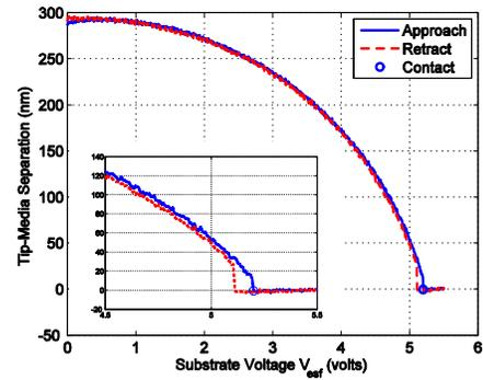
Fig. 6. A force/distance curve obtained by applying electrostatic force on the cantilever.
