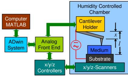
Fig. 2. Schematic of a single-lever data storage setup that serves as the development platform for a MEMS-based ultrahigh-density data-storage system.
