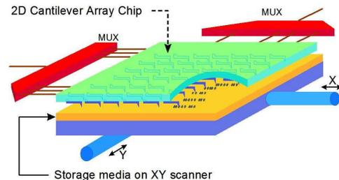
Fig. 1. Schematic of a MEMS based ultrahigh density data storage system.
