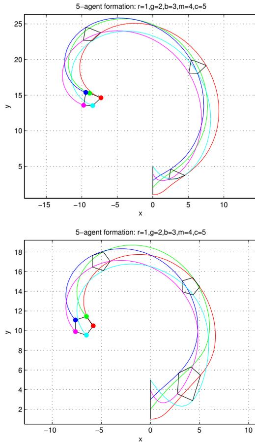
Fig. 4. Feedback disturbance in circular motion. Top: without compensator. Bottom: with compensator
