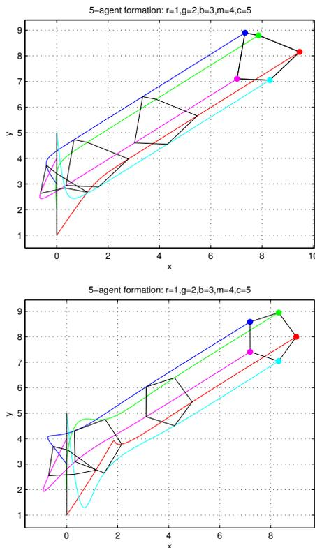
Fig. 2. Top: Agents do not achieve formation with feedback disturbance. Bottom: Agents achieve formation by using a compensator
