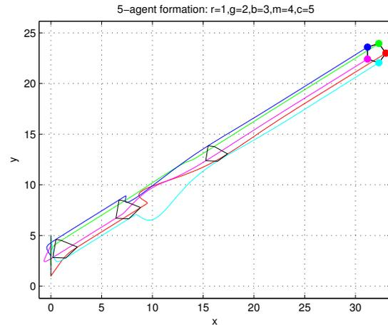
Fig. 3. Convergence with compensator. The first third is identical to the top plot of Fig. 2, but then the compensator is turned on.
