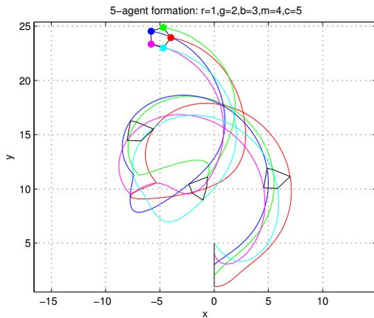
Fig. 5. Convergence while in circular motion. The beginning half of the path is identical to the top plot of Fig. 4. Then the compensator is turned on.
