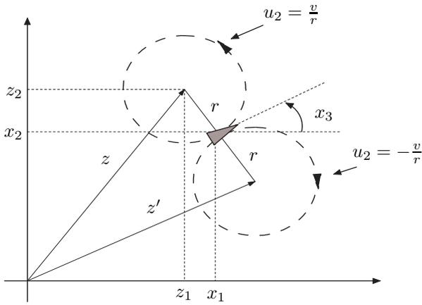
Fig. 1. Unicycle Circular Motion
