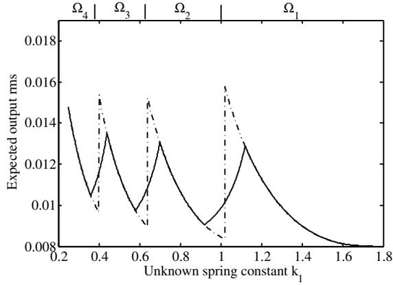
Fig. 3. Expected rms values for AMC (solid) and RMMAC (dash-dot) assuming perfect identification
