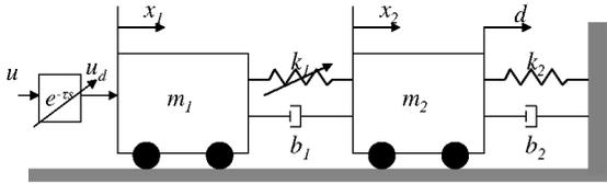
Fig. 2. The two-cart system possesses an unmodeled control delay, uncertain spring constant, process disturbance, and measurement noise.
