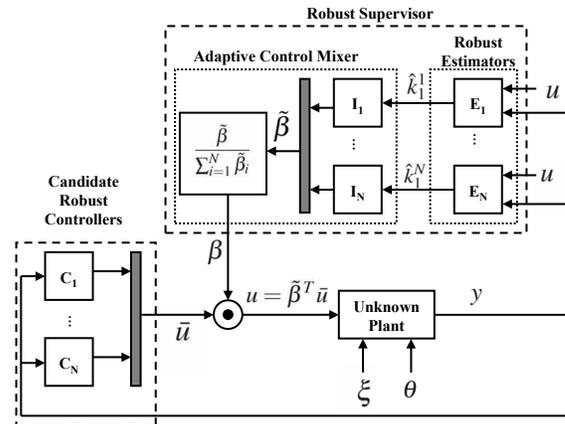
Fig. 1. The adaptive mixing control architecture
