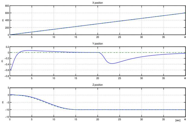
Fig. 3. Position  $x^i$ ,  $y^i$  and  $z^i$  (solid lines) with respect to the reference trajectories (dash-dotted lines).
