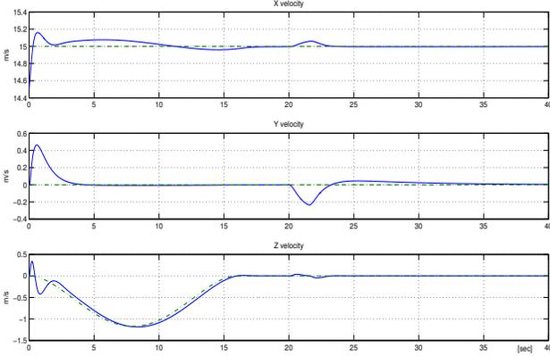
Fig. 4. Velocity  $x^i$ ,  $y^i$  and  $z^i$  (solid lines) with respect to the reference trajectories (dash-dotted lines).
