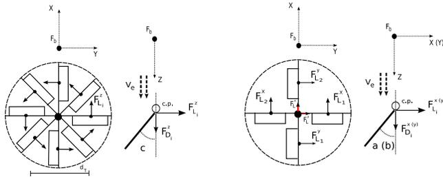
Fig. 2. Flaps subsystems: anti-torque and lateral/longitudinal flaps.
