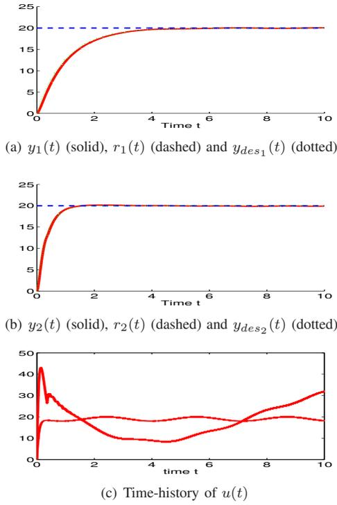
Fig. 1. Performance of  $\mathcal{L}_1$  adaptive controller for  $r = [20 \ 20]$
