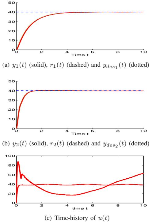
Fig. 2. Performance of  $\mathcal{L}_1$  adaptive controller for  $r = [40 \ 40]$
