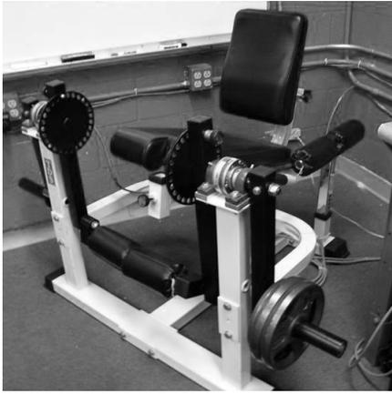
Fig. 2. Experimental testbed: Dual leg curl and extension machine.
