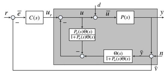
Fig. 1. The proposed DOB configuration (the shaded block) with an outer-loop controller  $C(s)$ . The signals  $r$ ,  $d$ , and  $n$  represent the reference command, the unknown external disturbance, and the measurement noise, respectively.  $y$  is the output of the closed-loop system while  $u$  is the feedback control to the plant.
