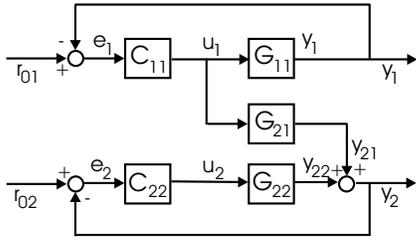
Fig. 1. Triangular control structure of a two-input/two-output system
