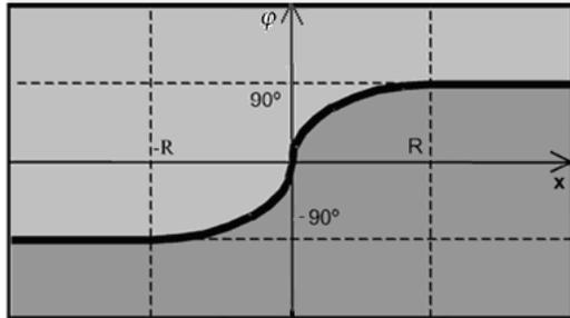
Fig.6. Steering angle  $\theta$  versus  $x$  and  $\phi$  for short paths. The dark color presents the  $\theta=-40^\circ$  and the light one presents  $\theta=40^\circ$ .
