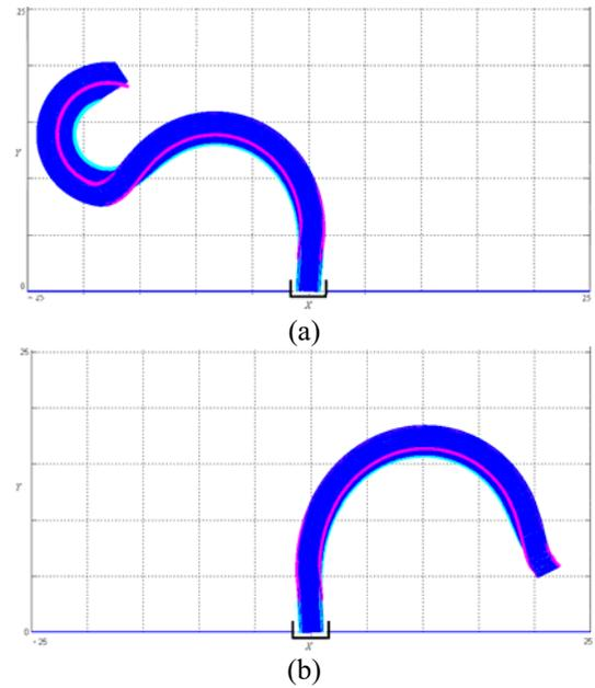
Fig.8. Simulated results of the parking maneuver corresponding to the initial configurations (a)  $x=-20$ ,  $y=18.4$ ,  $\phi=60^\circ$ ,  $t=93$  steps. (b)  $x=17.5$ ,  $y=8$ ,  $\phi=162^\circ$ ,  $t=86$  steps. [20]
