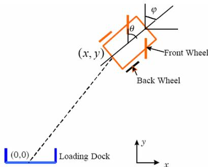
Fig. 1. Diagram of truck and loading dock.
