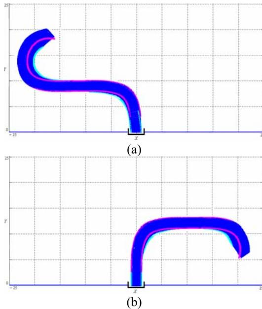
Fig.7. Results of the parking maneuver corresponding to the initial configurations (a)  $x=-20$ ,  $y=18.4$ ,  $\phi=60^\circ$ ,  $t=78$  steps. (b)  $x=17.5$ ,  $y=8$ ,  $\phi=162^\circ$ ,  $t=72$  steps.
