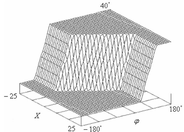
Fig. 5. Control surface of the fuzzy control system
