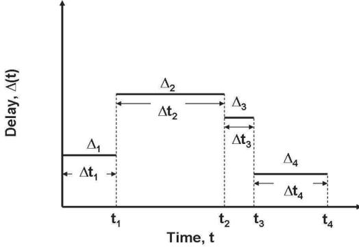
Fig. 1. Profile of time-varying delay.
