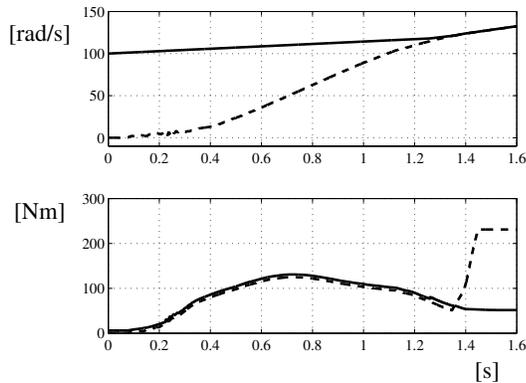
Fig. 8. Speeds ( $\omega_f$  continuous,  $\omega_c$  dashed) and torques ( $T_e$  continuous,  $T_{fc}$  dashed) time evolutions at vehicle start-up.
