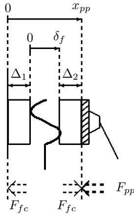
Fig. 3. A zoom of the axial displacement of the flat spring and forces on the friction surfaces:  $\delta_f = \Delta_f$  when the clutch is open and  $\delta_f = 0$  when the clutch is closed.
