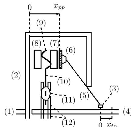
Fig. 1. A scheme of a dry clutch engagement system when the clutch is open: (1) crankshaft, (2) flywheel, (3) throwout bearing, (4) mainshaft, (5) diaphragm spring, (6) pressure plate, (7) friction pad on the pressure plate side, (8) friction pad on the flywheel side, (9) flat spring, (10) clutch disk, (11) torsional damper spring, (12) hub.
