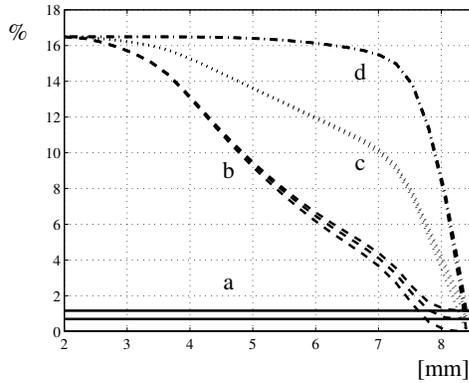
Fig. 7. Torque transmission relative percentage error of (20), (21) and (23) with respect to the nominal characteristic vs. throwout bearing position  $x_{to}$ : (a)  $r_i = R_1$  (continuous), (b)  $r_i(F_{fc})$  convex (dashed), (c)  $r_i$  linear (dotted), (d)  $r_i$  concave (dash—dotted).
