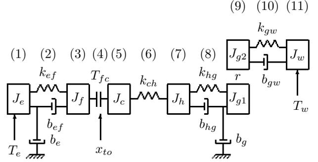
Fig. 2. A typical driveline scheme: (1) engine, (2) crankshaft, (3) flywheel, (4) equivalent representation for the dry clutch friction torque generation, (5) clutch disk, (6) damper spring, (7) hub, (8) mainshaft (hub-gearbox shaft), (9) gearbox and differential, (10) driveshaft, (11) wheels and vehicle.
