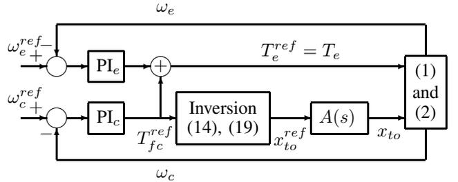
Fig. 6. A block scheme of the simulated AMT control system.
