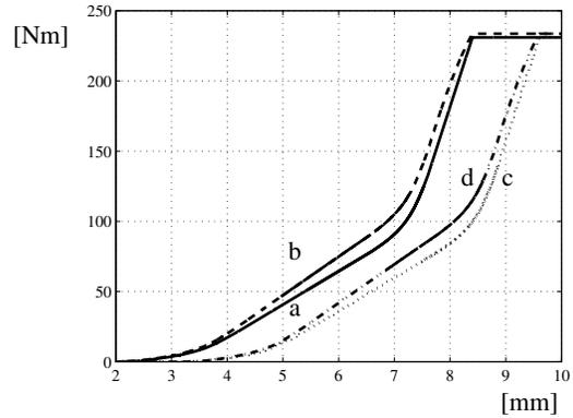
Fig. 9. Torque transmitted  $T_{fc}$  vs. throwout bearing position  $x_{to}$ : (a, c) nominal characteristic, (b, d) characteristic (20) with  $r_i(F_{fc})$  concave, (a, b) no wear, (c, d) in the presence of wear, i.e.  $\Delta = 5.7$ mm.
