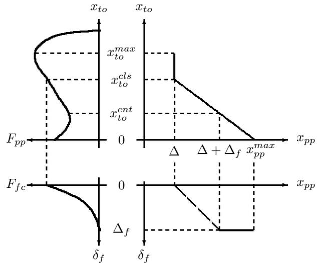
Fig. 4. Dry clutch characteristics. For a clutch engagement manoeuvre the plots should be intended by considering the following sequence of dependence:  $F_{pp}(x_{to})$ ,  $x_{pp}(x_{to})$ ,  $\delta_f(x_{pp})$  and  $F_{fc}(\delta_f)$ . When the clutch is mounted on the driveline  $x_{to}$  is constrained to be less than  $x_{to}^{max}$  which is the value of  $x_{to}$  corresponding to the maximum value of  $F_{pp}$ .
