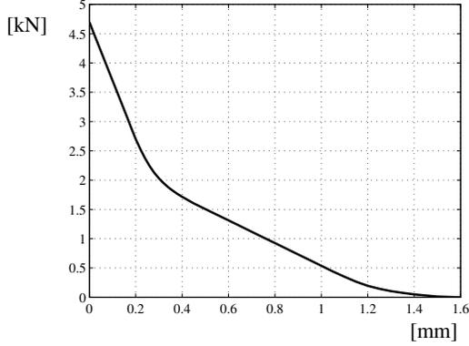
Fig. 5. Flat spring force vs. the flat spring compression:  $F_{fc}(\delta_f)$ .
